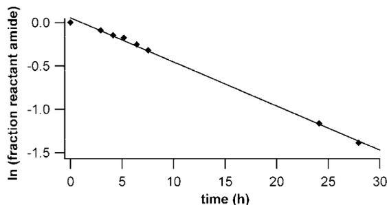
**FIGURE 2.** Plot of  $\ln$  (fraction reactant amide) vs time for the cleavage of amide **5** at pD 7.5.
