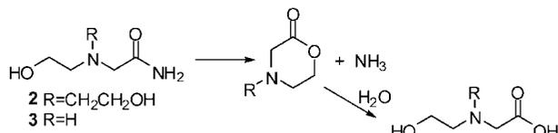
FIGURE 1. Hydrolysis of *N*-hydroxyethylamides.
